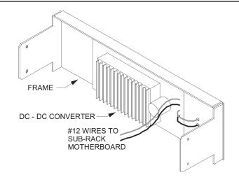
The DC to DC converters provide a regulated +13.8 Vdc to the output terminals over a wide range of DC input voltages. Valuable rack space has been saved by mounting the DC to DC converter inside the rear panel frame that attaches to the rear of the subrack. A terminal block is located on the outside of the subrack rear panel for the DC input voltage. The DC to DC converters comes in two different models.
