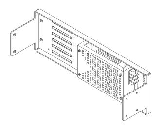
The PSA-12A09-PB-00 and PSA-12A09-UB-00 AC switching power supplies provide a regulated +13.8 Vdc to the output terminals. Valuable rack space has been saved by mounting the "PB" version AC power supply inside the rear panel frame that attaches to the rear of the subrack. The "UB" version is sold unmounted. An AC power socket is located on the outside of the subrack rear panel and accepts standard IEC320 type cordsets.
